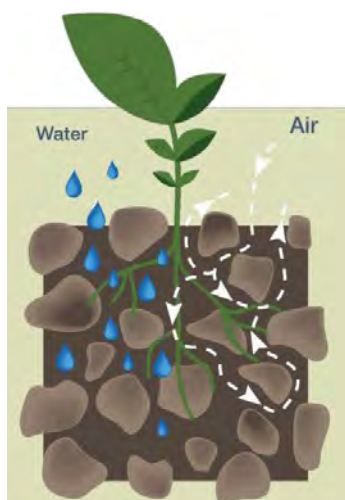
Figure 1. Good soil structure has adequate space (pores) between aggregates to alleviate compaction so that air, water and nutrients can reach plant roots.
